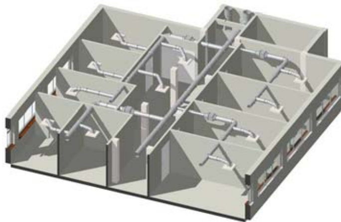
Figure 12 – 3D View of HVAC Ductwork (ArchiFM)
